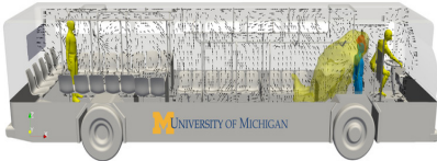
Numerical model showing the flow of air and concentration of aerosols inside a campus
